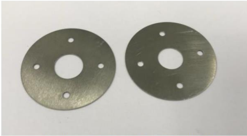
Fig. 2. Photograph of the machined line standards for the WR-5 band MCK. Both lines have the same thickness of 0.420 mm. The diameters of the inner holes are 9.052 mm and 8.200 mm.
